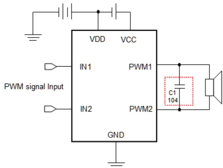
\* If voltage is higher than 6.0V, C1 (0.1uF) is necessary for endure high voltage.
